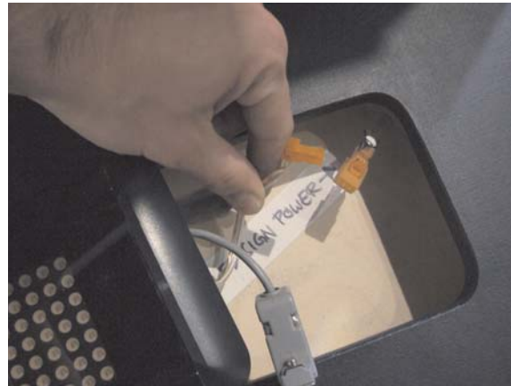
The orange connection is the power connection. You have to push a tiny clip on the plug to disconnect plug and socket.
