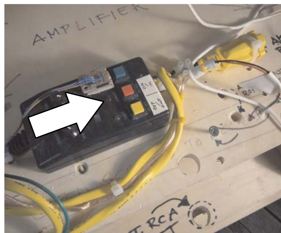
The remote control of the fog machine: Check if the red LED is bright (arrow) Are all the buttons in correct position?
