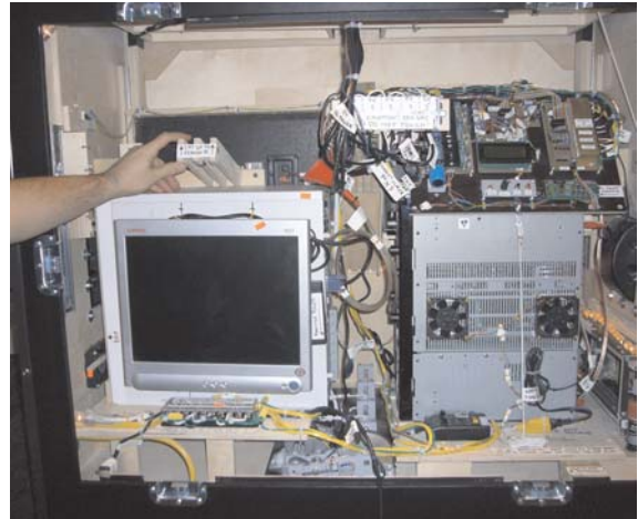
The wooden clasp holds the PC with a magnet in position. It can only be lifted up, if the light effects stage is lifted up as well.
